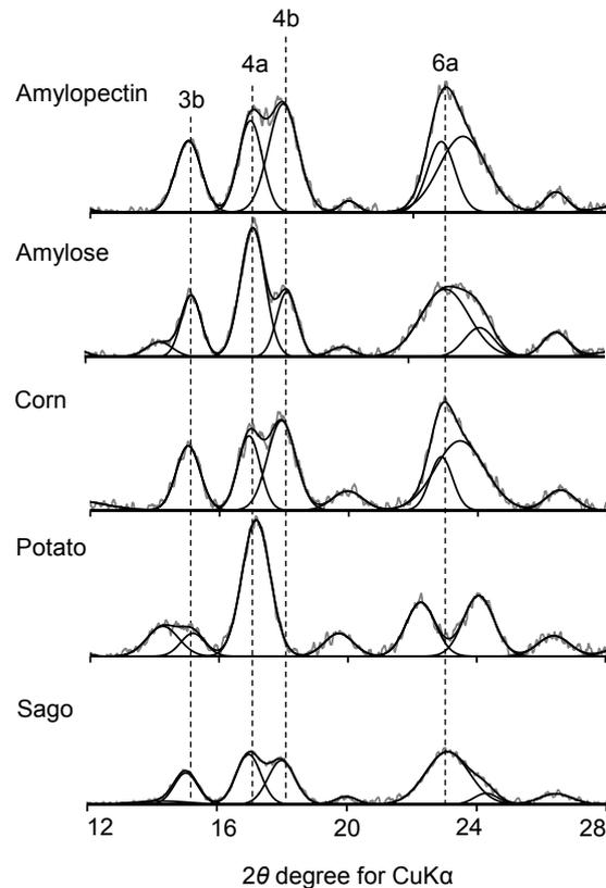
**Fig. 2.** X-ray diffraction after wave-form separation
