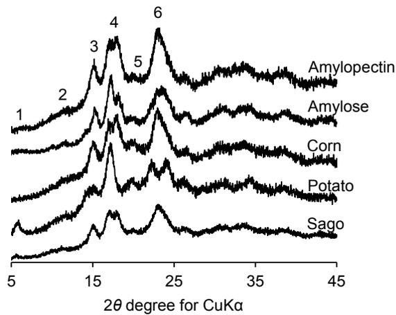
**Fig. 1.** X-ray diffraction patterns of sago starch
