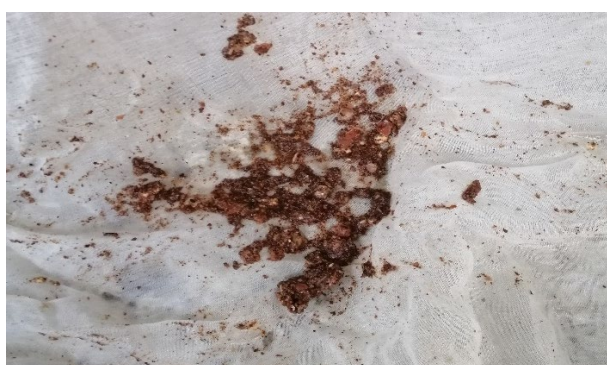
Fig. 1 Impurities washed out and collected on a 100-mesh sieve from starch sold at Lorengau market.
