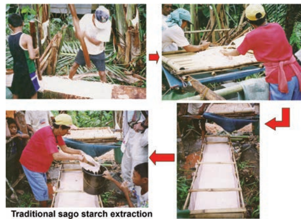
Fig. 2. Wet-extraction method for sago starch
