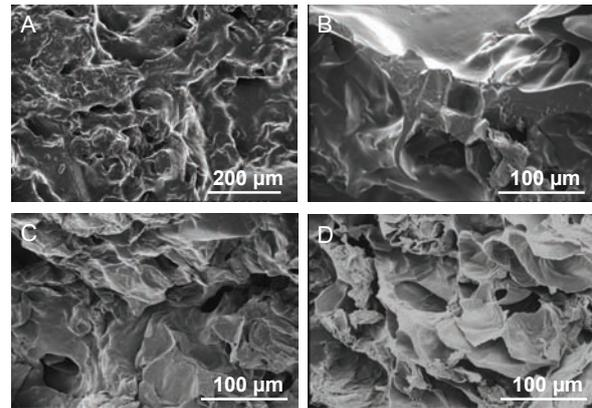
**Fig. 2.** Scanning electron micrographs of foam prepared from sago residue A, Surface of foam from native sago residue; B, cross section of foam from native sago residue; C, surface of foam from acid-treated sago residue; D, cross section of foam from acid-treated sago residue
