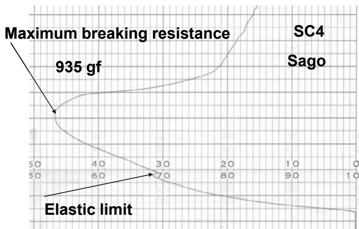
Fig. 2. Maximum breaking resistance of sago leaflet samples
